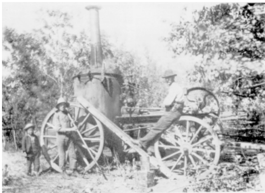
A “Prips Kjaetle” an upright steam engine mounted on a wagon which could be moved from village to village. These units were found in the East Reserve by 1878. This “Prips Kjaetle” owned by Cornelius F. Broesky, Schönenberg, was an antique by the time this photograph was taken. Photo courtesy of Grunthal History, page 53.
