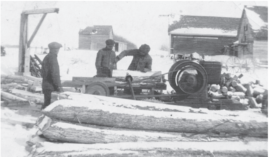
The Plettville businesses included a home-built firewood and feed crushing unit which travelled around the neighbourhood. Here the unit is cutting firewood on the Plattebof. View to the east. The north ends of the scheune and bogbarn, right, and the old granary, moved out from the Blumenort village, middle rear. Jakob R. Plett, middle. In 1946 the Jakob R. Plett house was built to the left of photo. Jakob R. Plett, middle, operated the unit. Photo - Jakob R. Plett, 1930.
