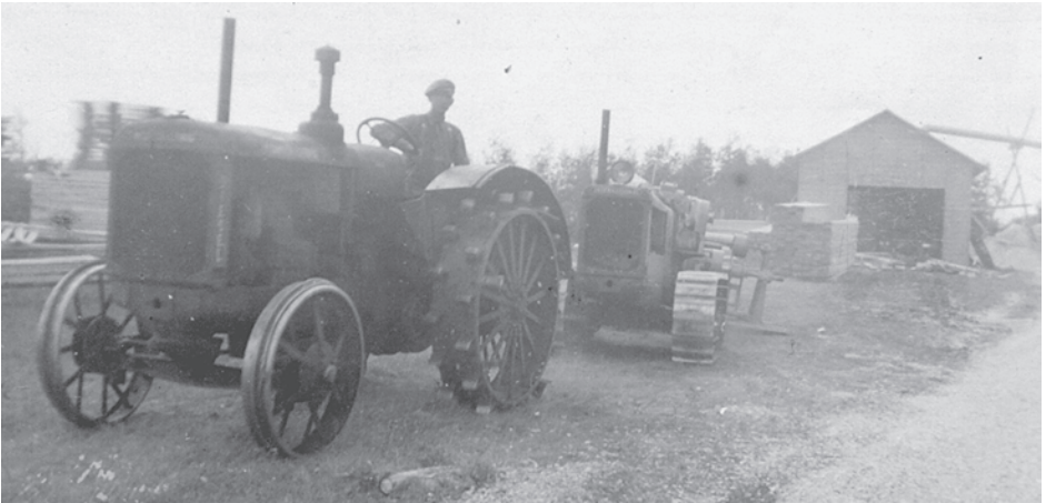
Above: Roblin planing operation, 1942. The TD35 is being pulled started by the WD 40. The tractor operator may be Cornie Fast. The TD 35 was started on gas and then switched to diesel. It was a poor starter.
