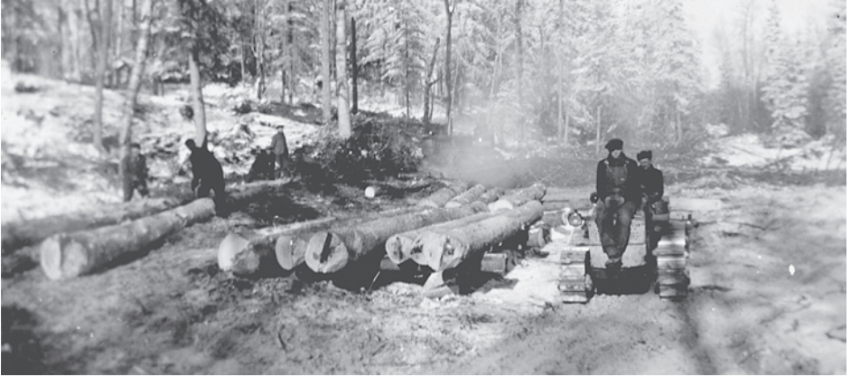
The trees were skidded out of the forest to landings where they were bucked up into logs. From the landings the logs were hauled to the sawmill site by crawler and sleigh or loaded onto trucks and hauled to the sawmill. Here they were stockpiled and eventually sawed into lumber. Photo - Nettie Fast.
