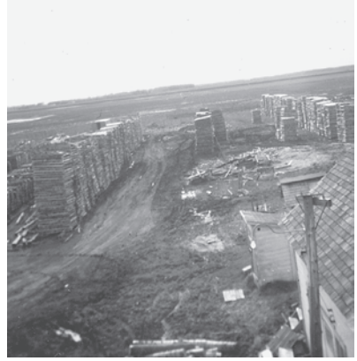
After the poplar logs were cut up, the boards were piled for drying. The lumber storage area, view to west from the second floor saw mill in the woodworking shop. In the distance, is the oak bush on SE28-7-6E, where grandfather Peter R. Reimer and later his son David P. Reimer lived. Photo - George R. Plett.
