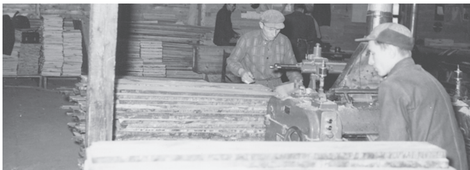
Surface planer, planes boards to even thickness. Peter Wiebe (middle) and Levi K. Reimer (right).
