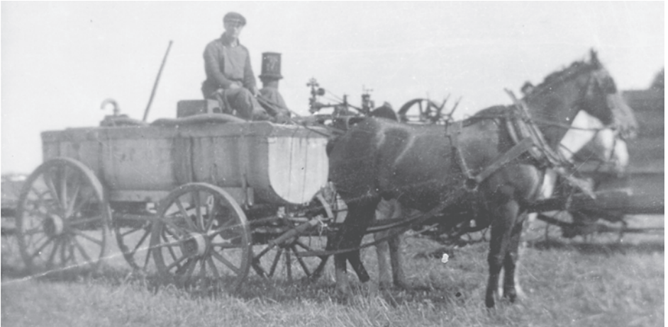
The water wagon was an important element of the threshing outfit, supplying water both to the threshing workers and horses, as well as for steam engine boiler.
