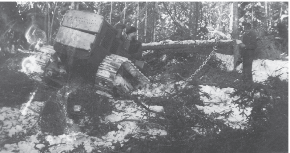
Below: Abramam R. Plett's gas-burning Catepillar 22, snaking a tree out of the forest. Operator, son Henry K. Plett. Photo - Nettie Fast.
