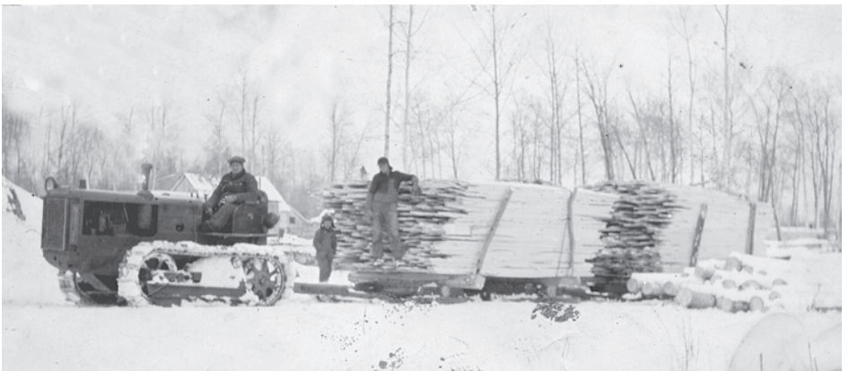
Around 1938 Plett & Co. acquired a TD35 International crawler for their lumbering operations, also used for brush plowing during the summer season. Jakob R. Plett is driving the cat hauling two sleighs full of saw lumber to the railway siding in Vassar. The regular operator in Vassar was Abram A. Reimer (Abr. P.). Photo - Jakob R. Plett.
