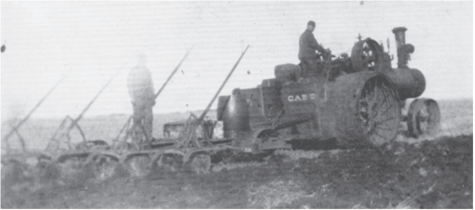
Case 25/75 steam engine and eight bottom gang plow. Plowing stubble two miles west of Twin Creek (Neuanlage) in 1919. Engineer is John P. Reimer and fireman (bent over) is Cornelius R. Plett. Man on gang plow unidentified. Photo - Peter P. D. Reimer/Plett Picture Book, page 150.
